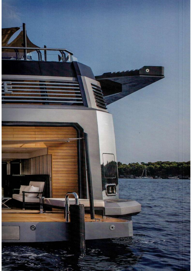
There is abundant use of stainless steel inside and out, and removable stanchions custom made of steel with a painted fibreglass finish. Aligning the polished stainless steel plates on the bow and the hull railings around the helipad, and joining the stainless steel details to materials on the inside, were some of the biggest challenges for CRN's workforce.
