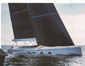
CANOVA Baltic Yachts // 43.3m Regeneration of energy under sail // Battery-electric propulsion charged by generators
