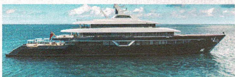
LONIAN Feadship // 87m // Diesel-electric battery hybrid // Zero-emission operations possible
